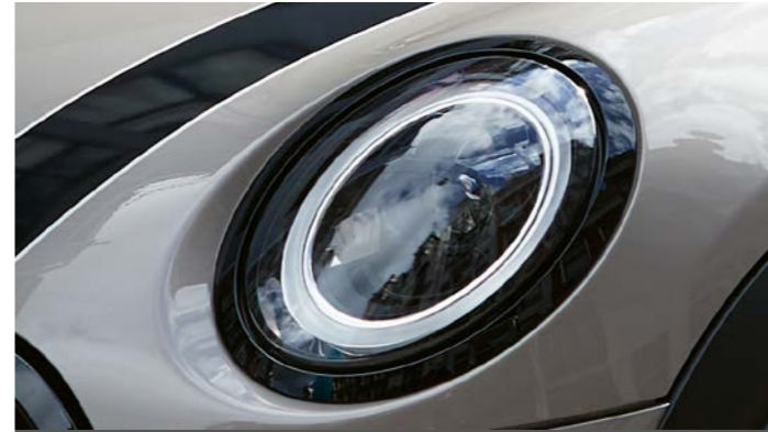
Adaptive LED headlights with Matrix function 9
